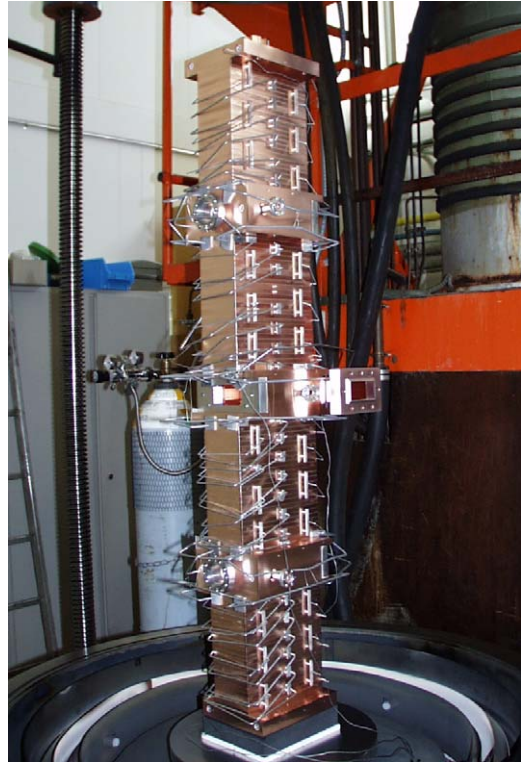
Fig. 13. The module placed vertically in the oven.
