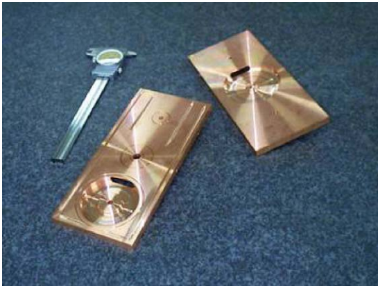
Fig. 11. Half-cell plates showing a coupling half-cell (left) and an accelerating half-cell (right). Note the coupling slot.
